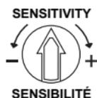
**Setting Sensitivity:** The dial is similar to a clock. The factory setting of the condensation (humidity) sensitivity dial is set to the noon position. If you feel the factory setting is too slow in turning on your fan, turn the dial to the right an hour at a time. Or, if you feel the factory setting turns your fan on too quickly, turn the dial to the left an hour at a time until the desired sensitivity level is reached.
